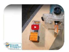
The acrylic can be routed by first fully supporting the product marking the trim line where required, and then using a guide to trim along the edge in a smooth and fluid motion.
